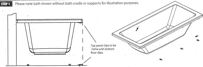
Using a cross headed screwdriver secure the bath panel clips to floor and the underside of the bath using the screws provided. Ensure that the panel clips are equally spaced and are in line with each other top to bottom and that the clips are marginally proud of the bath rim.
