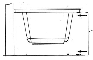
Please note to allow for future access the clips are designed to hold the panel not lock it into position.
